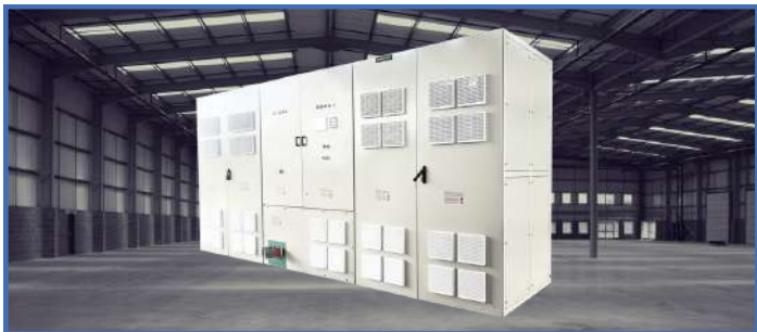
1.43 MW Rectifier—indoor free-standing panel type— for Zero Footprint Industries, Moradabad (328V, 4350A, SCR-controlled)
