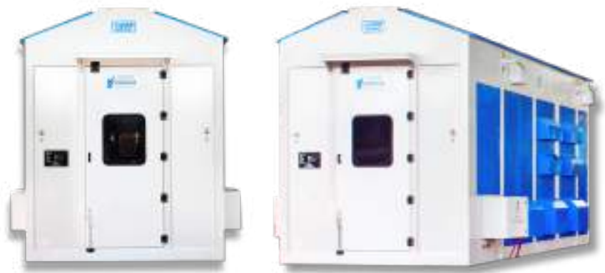
2x558kW Rectifiers Containerised - 3600A/ 155V - Commissioned at NTPC, Leh Green Hydrogen Mobility Pilot Project (Forced Air-Cooled; Outdoor Container Type)
